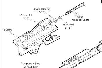
• As a temporary stop, insert a screwdriver into the hole in the front end of the T-rail.
